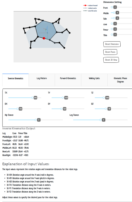
Fig. 4. Visualization of leg configuration obtained from inverse kinematics.
